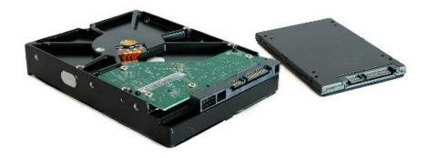
Your hard drive's capacity is measured in units called bytes. A single byte is large enough to store one character of text. These days we use gigabytes, which are one billion bytes. Hard drives range in size, but newer computers typically offer 128-512 gigabytes of storage. We suggest at least 250 gigabytes of HDD storage, or 128 gigabytes of SSD storage.
