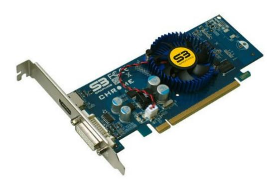
GPU's are often built into a computer's motherboard or integrated into its CPU. For those with a need for extra power, graphics cards (pictured above) are an option. They are a separate component that fits into your motherboard via an expansion slot.
