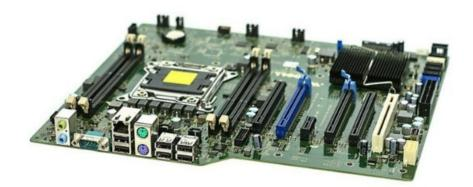
The motherboard is typically located under the keyboard of a laptop computer. On a desktop computer, it is mounted on the left or right interior side of its case. They are not universal. Often, they are designed with specific types of devices and components in mind.
